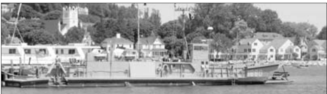
The LCU 1680, a Navy Reserve vessel out of Buffalo, New York, docked on Mackinac Island from June 22 to 24 as part of a training exercise for its crew of 18. The boat has a flat bottom and the unique ability to cruise right up to a beach and unload soldiers and supplies.
